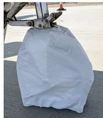
CJ1 Nose Gear Tire Cover, test fit
