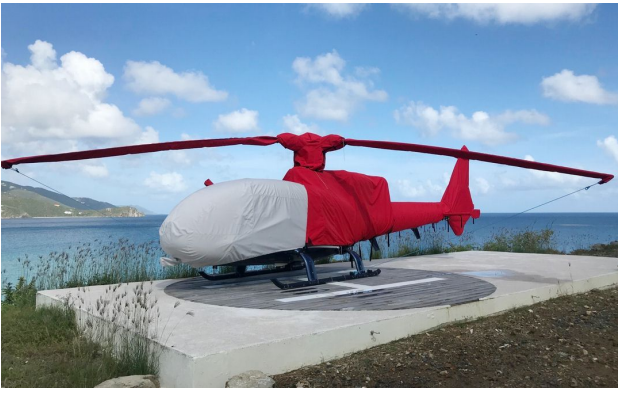
Aerospatiale AS341/342 Gazelle Full Cover Set Aerospatiale Gazelle AS341 Bubble, Rotor Mast, Blade, Engine & Tailboom Covers (some are test fit covers)
