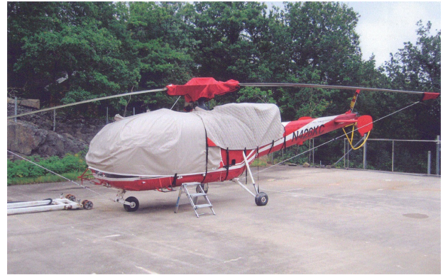
Alouette III Rotor Hub Cover & Engine/Transmission Cover Alouette III Bubble, Rotor Hub & Engine Covers, Blade Tie-Downs
