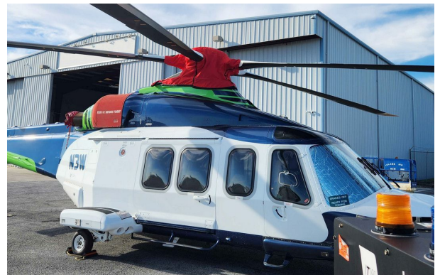
Agusta AW139 Rotor Mast Cover, covers upper deck & aft of rotor mast area
