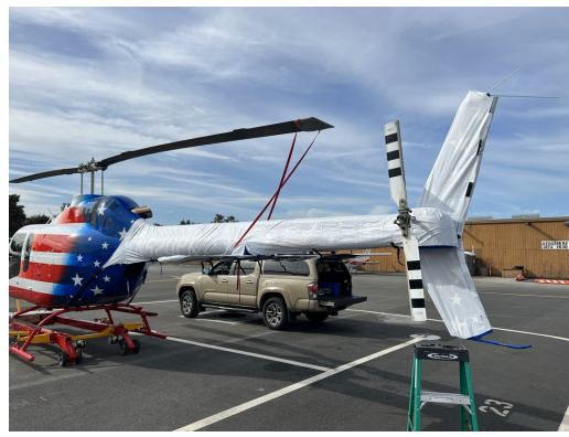
Bell 505 Tailboom & Stabilizer Covers, test fit cover
