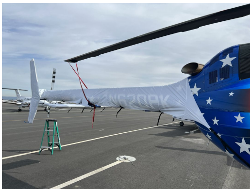
Bell 505 Tailboom & Stabilizer Covers, test fit cover
