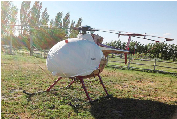
MD500D Bubble Cover with Intake Add-On
