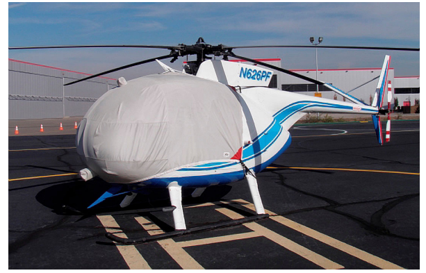
MD500C Bubble Cover with Wire Strike detail
