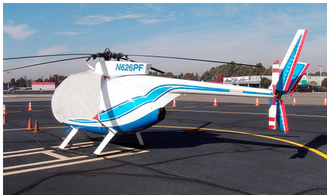
MD500C Bubble Cover with Wire Strike detail
