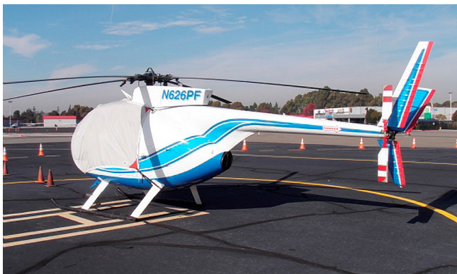
MD500C Bubble Cover with Wire Strike detail
