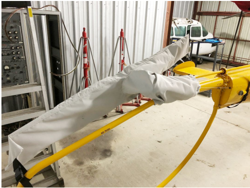
Enstrom F280 Tail Rotor Cover
