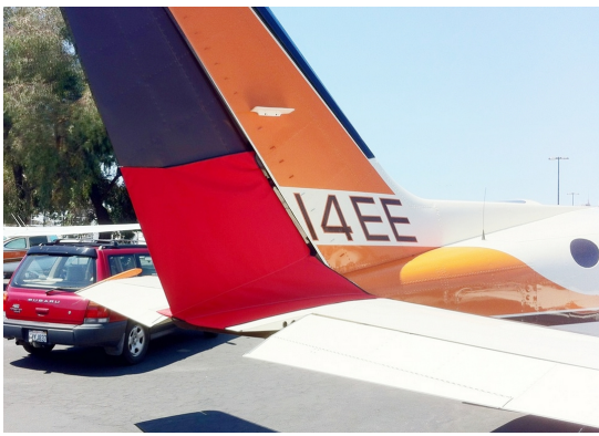
Cessna 414 Rudder Openings Cover (bird barrier)
