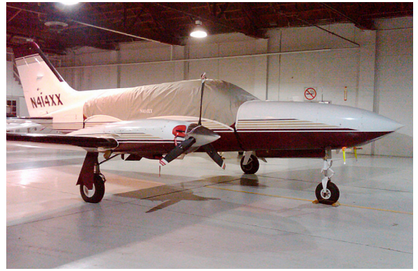
Cessna 414 Canopy Cover and Engine Inlet Plugs
