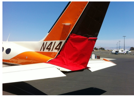
Cessna 414 Rudder Openings Cover (bird barrier)
