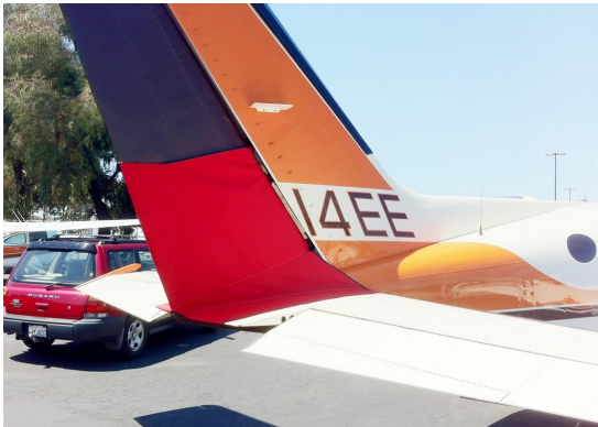
Cessna 414 Rudder Openings Cover (bird barrier)
