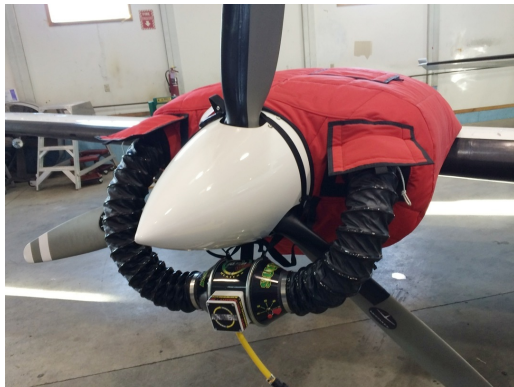
Cessna 402 Insulated Engine Cover with Heater
