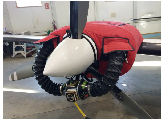
Cessna 402 Insulated Engine Cover with Heater
