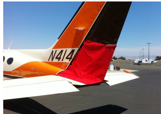
Cessna 414 Rudder Openings Cover (bird barrier)
