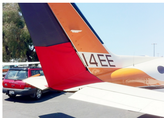
Cessna 414 Rudder Openings Cover (bird barrier)
