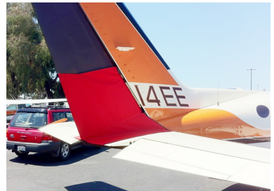
Cessna 414 Rudder Openings Cover (bird barrier)
