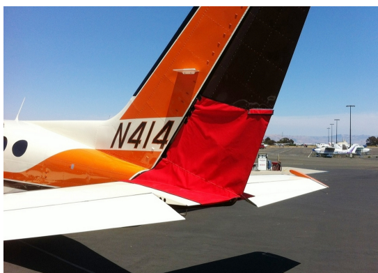
Cessna 414 Rudder Openings Cover (bird barrier)
