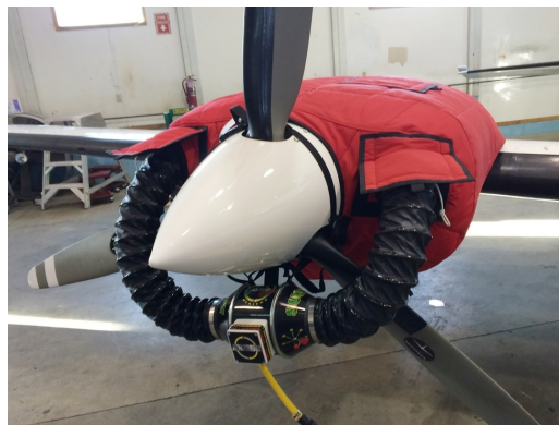
Cessna 402 Insulated Engine Cover with Heater
