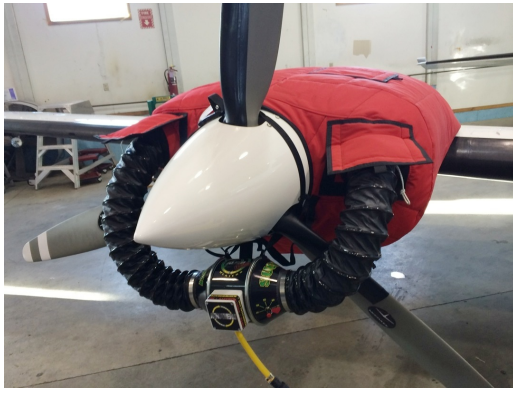
Cessna 402 Insulated Engine Cover with Heater
