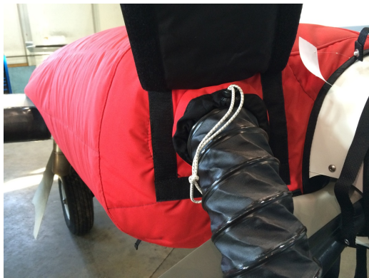
Cessna 402 Insulated Engine Cover with Heater
