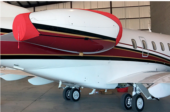
Canadair Challenger 300 Intake/Exhaust Covers, 3-Strap Intake/Exhaust Covers, 3-Strap Type. Successfully installed by two crew, one ladder.
