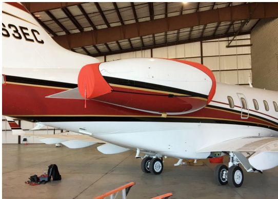
Canadair Challenger 300 Intake/Exhaust Covers, 3-Strap Intake/Exhaust Covers, 3-Strap Type. Successfully installed by two crew, one ladder.
