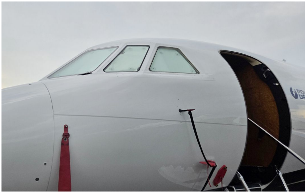
Dassault Aviation FALCON 2000EX Cockpit Heatshields (set of 7) Dassault Aviation FALCON 2000EX Cockpit Heatshields (set of 7)
