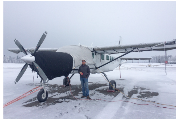
Cessna 208 Caravan Insulated Engine, Cockpit & Wing Covers
