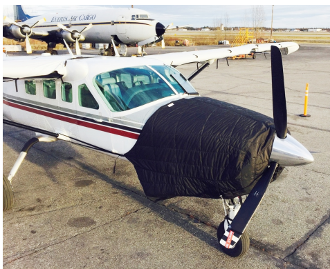
Cessna 208 Caravan Insulated Engine Cover, fully enclosed
