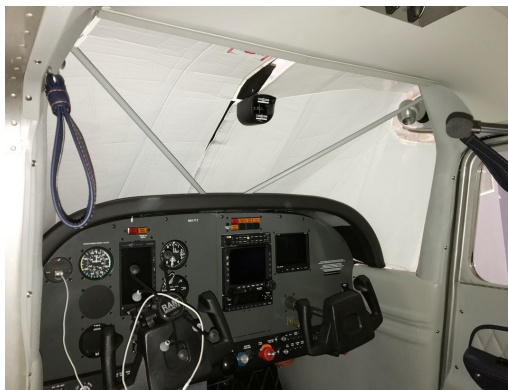
Cessna 180 Skywagon Windshield Heatshield, (W/ Compass)
