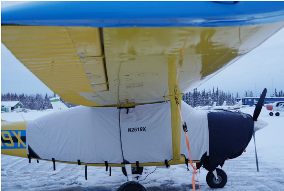
Cessna 206 Extended Canopy Cover, Insulated Engine Cover
