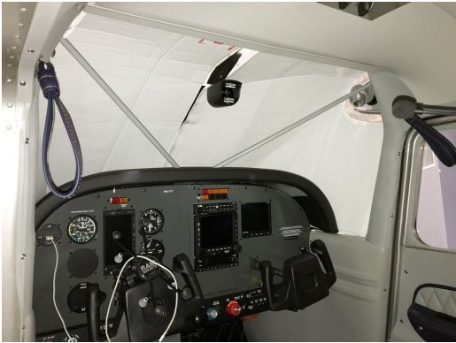
Cessna 180 Skywagon Windshield Heatshield, (W/ Compass)
