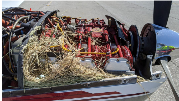
Engine and Oil Cooler Inlet Plugs ENGINE PLUGS PREVENT BIRD NEST FOD. Piper Saratoga Engine Cowling Bird's Nest
