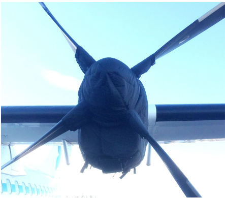
ATR-72-202 Insulated Engine & Prop Hub Covers
