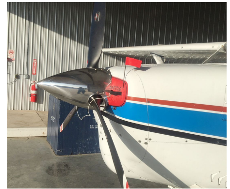
ENGINE PLUGS PREVENT BIRD NEST FOD. Piper Saratoga Engine Cowling Bird's Nest Cessna 210 Inlet Plugs, early model
