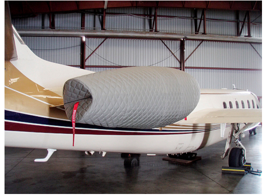
IAI Westwind 1124 Insulated Engine Nacelle Cover
